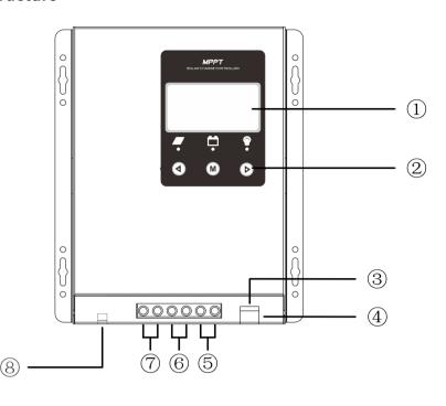
①LCD Display Screen ②Button ③Communication port ④Grounding terminal
