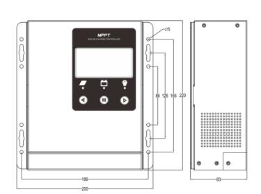
40A dimensions: Mounting hole pitch: 86mm\*186mm Mounting hole pitch: 126mm\*186mm Mounting hole pitch: 166mm\*186mm Mounting hole diameter: Φ5mm Length\*Width\*Thickness: 220mm\*200mm\*83mm
