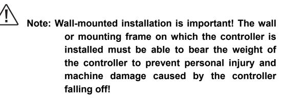
The controller is required to be perpendicular to the mounting surface, If the installation angle deviates from the vertical direction by more than 45 degrees, it will cause poor heat dissipation of the controller, which may affect the power output of the controller.
